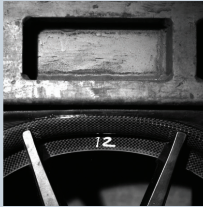
Composite wheels demonstrate up to 1600 joules when toughened Araldite® resin is used
